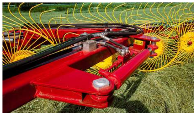
Hydraulic cylinder for transport position.
